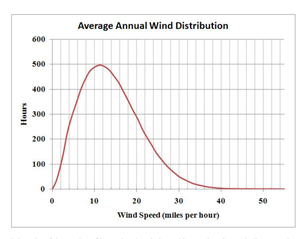
It is a plot of the number of hours that the wind speed is at a given interval. For example, of the 8760 hours in a year, the wind will be at the 15 mph interval for 450 hours (roughly 5% of the time). As one would expect, the very high wind speeds would exist for only a few hours. When the hours at each interval are added together, they total 8760 hours.
